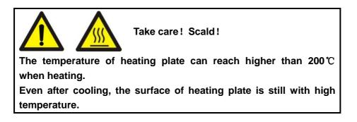
The sealing quality, to some extent, depends on the maintenance of heating plate and silicon strip.
